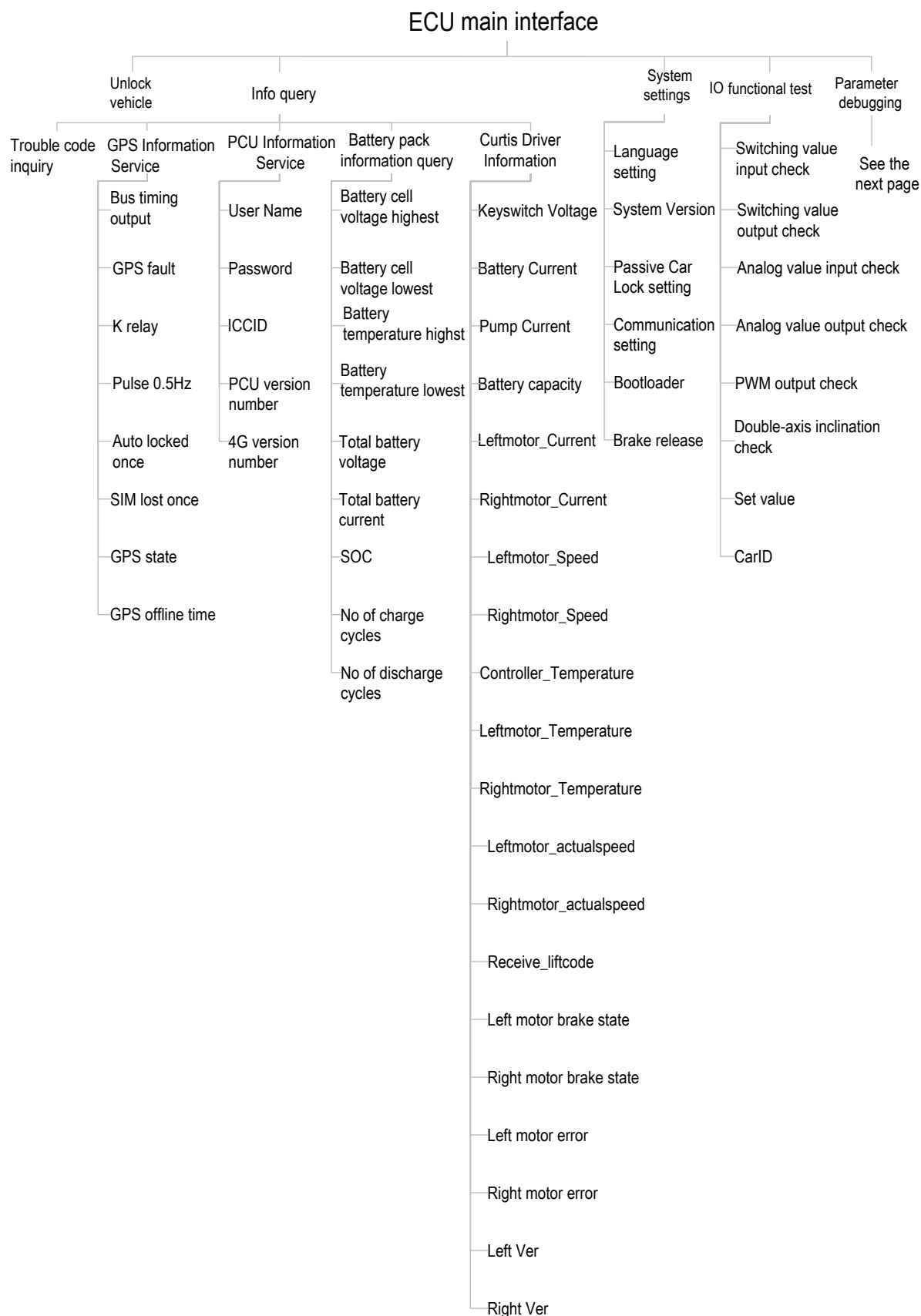
Figure 6-16 System interface description
