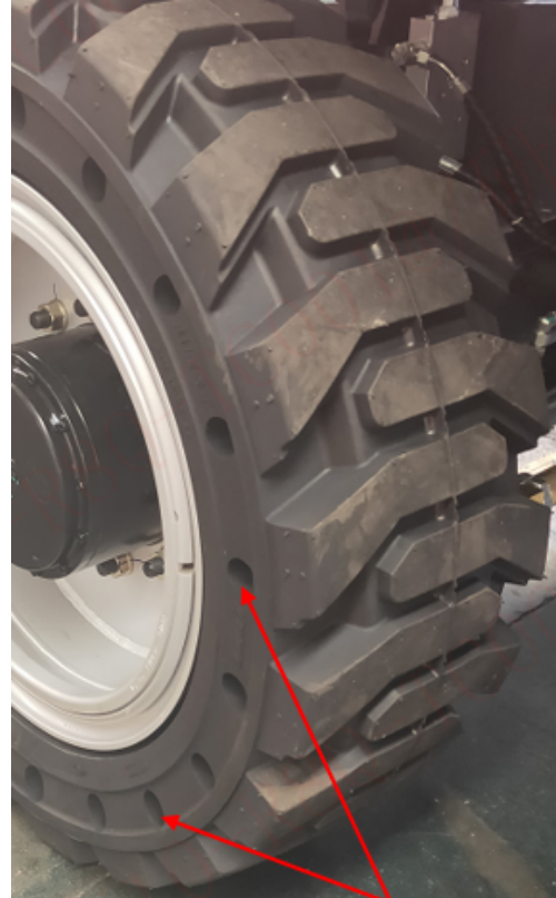
Figure 7 Trous de ventilation
