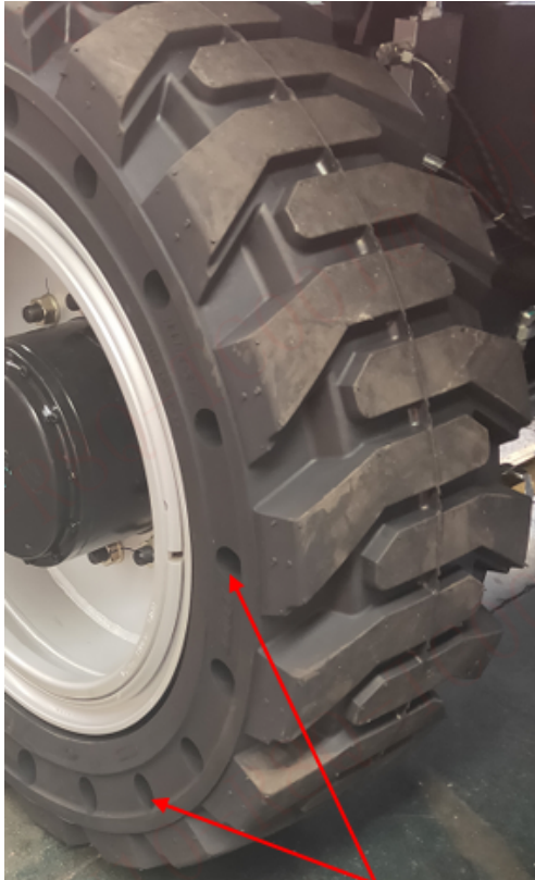
Figure 4 Trous de ventilation
