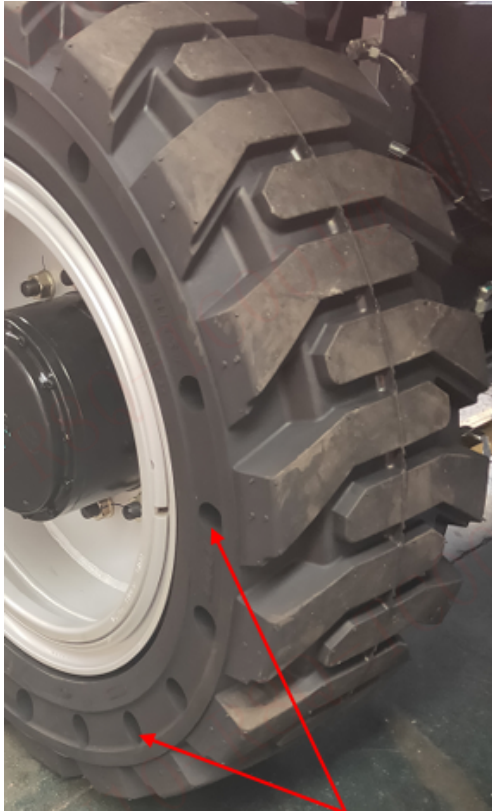
Figure 4 Trous de ventilation
