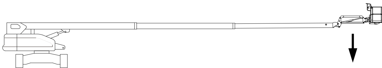
Fig. 2 Position of lowest forward stability of the machine
