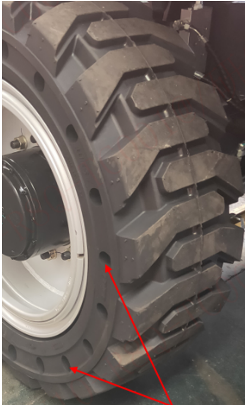
Figure 4 Trous de ventilation
